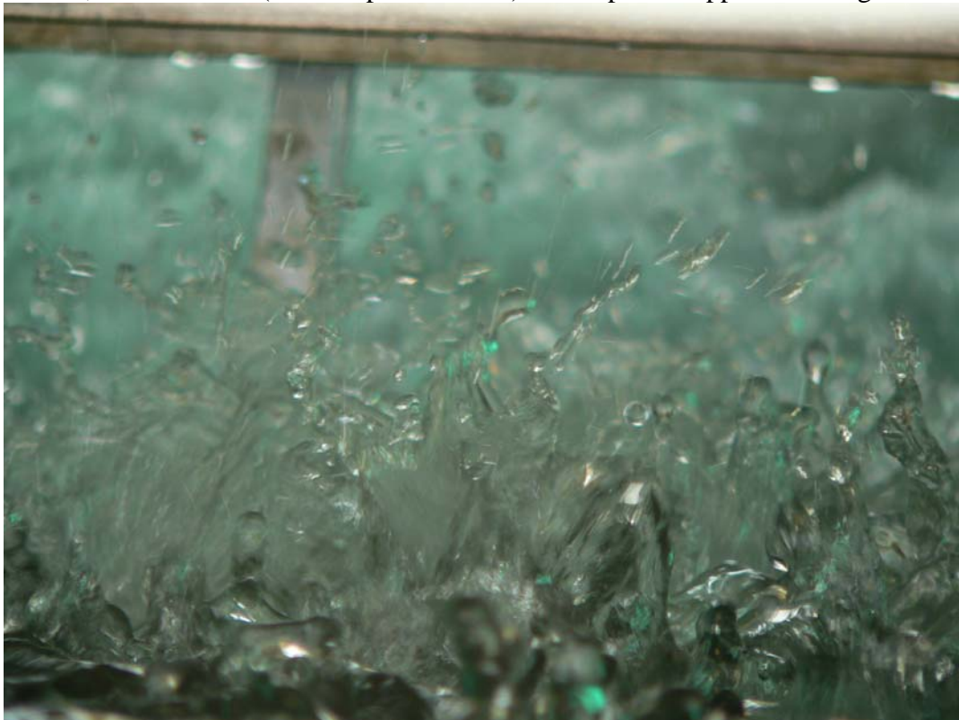
Fig. 7-3 - High-speed photographs of water droplets in ballistic trajectory, viewed from upstream - Skimming flows, h = 0.1 m, \theta = 21.8^\circ
