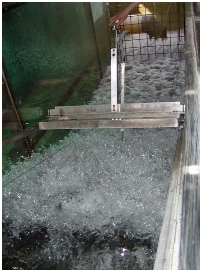
(B) Looking downstream at the trolley system supporting a double-tip conductivity probe - d_c/h 1.33, Re = 4.7 E+5
