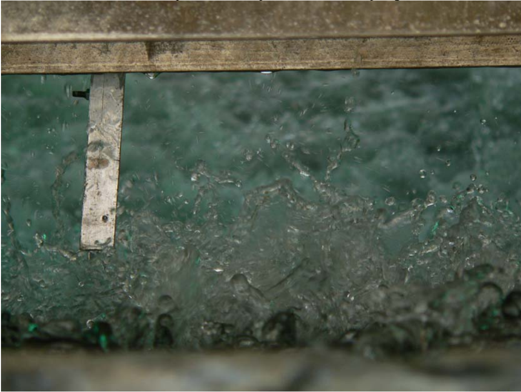
(A) d_c/h = 1.33 , Re = 5.7 E+5 , shutter speed: 1/320 s, probe located at step edge 7
