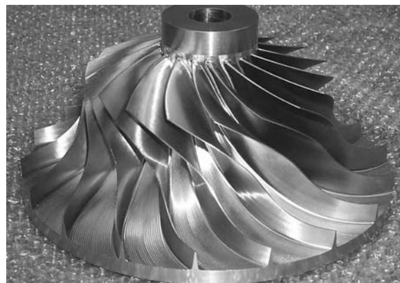
■ FIGURE 12.33 Centrifugal compressor rotor. (Photograph courtesy of concepts NREC.)
