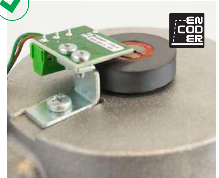
Check on the movement of motor by encoder which guarantees precision and safety
