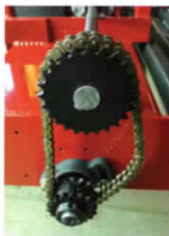
Figure #20 CHAIN INSTALLED, READY FOR SECOND CHAIN
