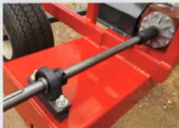
Figure #27 DRIVE SHAFT AND BEARING COMPLETELY INSTALLED
