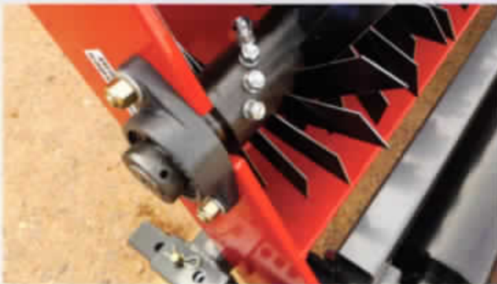
Figure #32 BLADES AND RETAINER BOLTS (INSTALLED)
