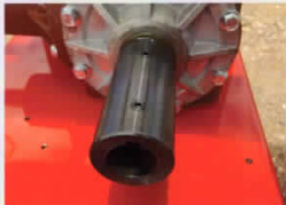
Figure #25 GEAR BOX WITH SHAFT COUPLER INSTALLED
