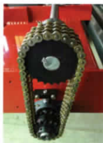
Figure #21 BOTH CHAINS INSTALLED AND TENSIONED
