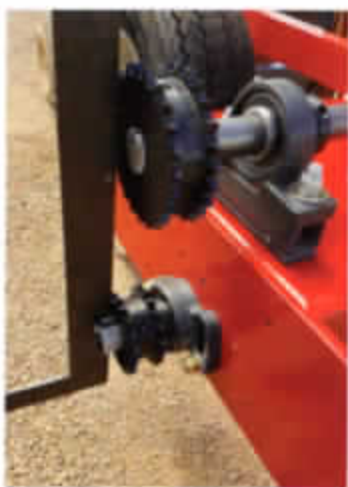
Figure #18 & #19 SPROCKET ALIGNMENT USING A SQUARE
