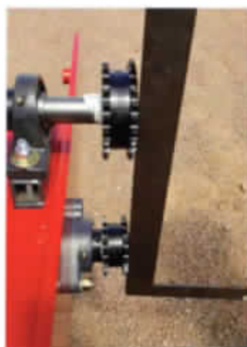
Figure #18 & #19 SPROCKET ALIGNMENT USING A SQUARE
