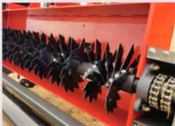
Figure #45 NEW CUTTING BLADES INSTALLED (NOTE DIRECTION OF BLADES)
