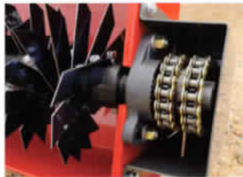
Figure #37 SLOTTED REEL BEARING BLOCK, CHAINS AND SPROCKETS (INSTALLED)
