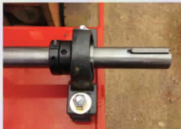
Figure #26 BEARING, DRIVE SHAFT, LOCKS AND KEYWAY INSTALLED
