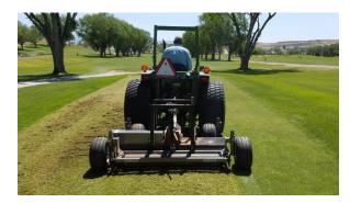
Cutting depth is adjustable from 0" to 2" with a simple ratchet mechanism. Often after renovation is complete and excess thatch is removed, the field can be used immediately. One tractor and a operator can recondition a football field in 2-3 hours.
