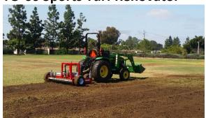
Renovate, vertically mow, dethatch, and slice aerate turf all at the same time.
