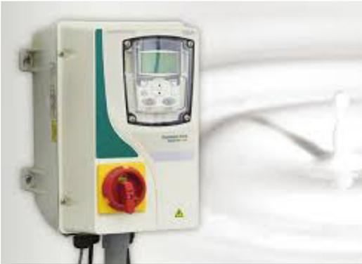
The KonstantKool variable speed control provides the operation of the milk pump by regulating the speed of the pump based on the level of milk in the receiver or milk/wash reservoir. A continuous, slow delivery of milk through the filter and to the plate cooler also provides a more thorough
