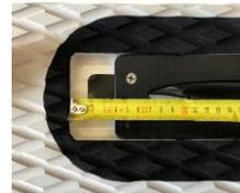
\* Clew position Jib is the position of the shackle on the clew board.
