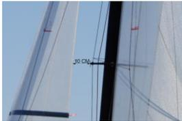
\* The jib car should be positioned at the center of the numbers indicated on the self-tacker Nacra sticker.
