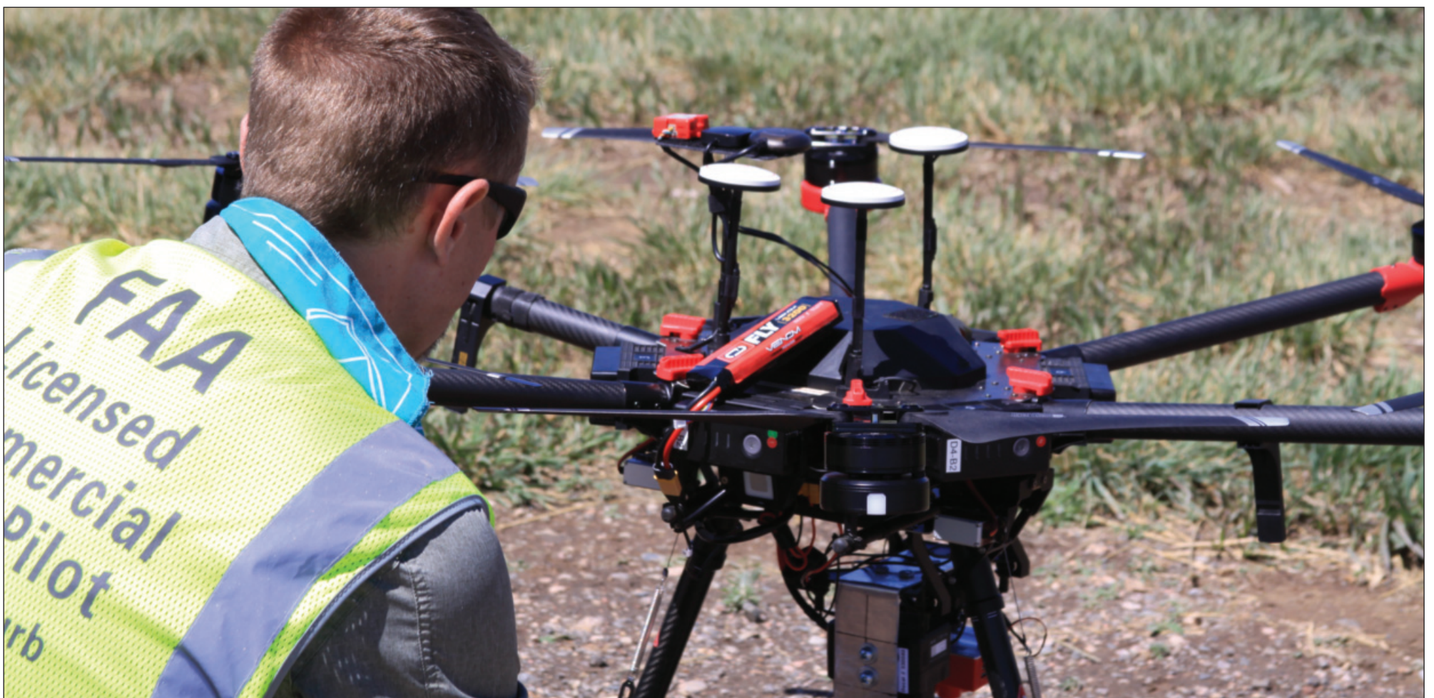
Christopher Robertson, director of the CSU Drone Center, conducts a pre-flight inspection of a $5,000 DJI Matrice 600, a 22-pound professional drone with broadcast quality.
