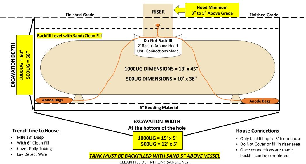
NO ROCKS, NO FRACTURED STONE/CRUSH, NO MATERIAL WITH SHARP EDGES. (THESE WILL SCRATCH THE PROTECTIVE COATING AND CAUSE PREMATURE TANK FAILURE) 500UG - 5-7 YARDS OF FILL , 1000UG 8-10 YARDS OF FILL
