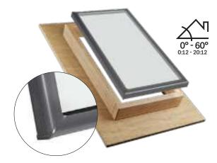
Curb-mounted skylights are the most common installation preference in low-pitch or flat-roof situations. The "curb" is a frame built mostly of two-by-fours that are attached to the roof. The skylight is then installed on top of the curb. You can imagine it as a shoebox: the curb is the box and the skylight is the lid.
