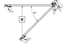
The free exit **H** is the minimum perpendicular distance from the bottom frame to the insulating glass unit.
