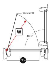
The free exit **W** (radius) is the minimum perpendicular distance from the side frame to the opposite side sash.
