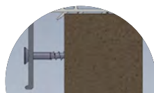
Use fasteners at each pre-drilled location in the frame.
