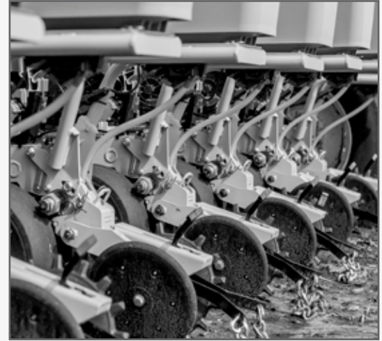
LASERPRO1 w/ vDrive insecticide boxes Integrated with FurrowJet.
