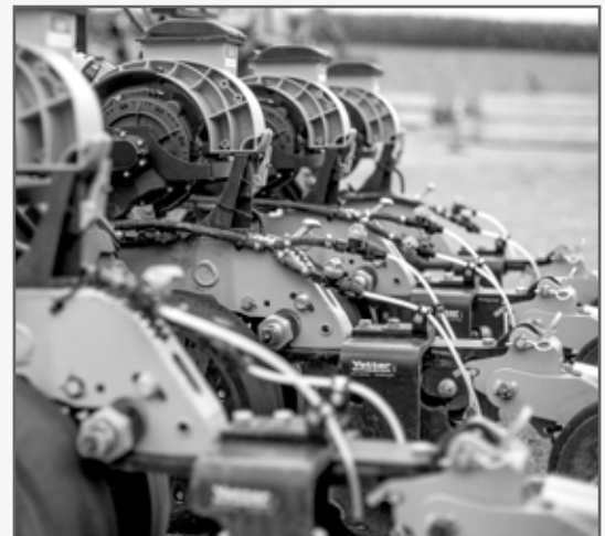
Designed for custom configuration Dealer-installed vSet seed meters, SureDrive, & fertilizer openers.
