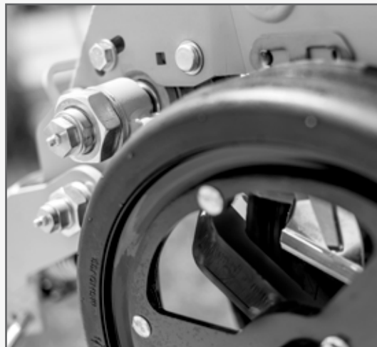
Lateral & Built-In Camber Gauge Wheel Adjustment Standard tungsten carbide disc scrapers offer extended wear
