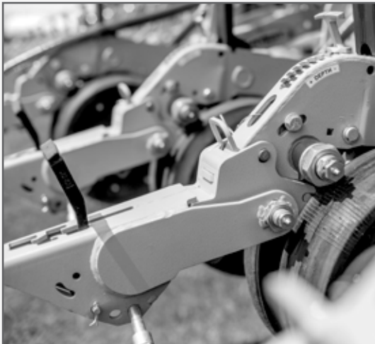
QUICKRELEASE™ CLOSING WHEEL MOUNT Pull a pin for fast service or swapping mounts w/ different style wheels
