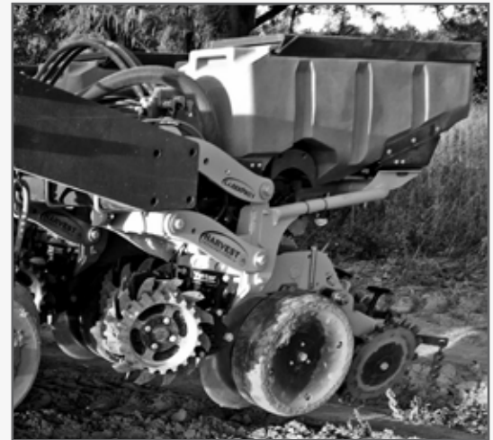
LASERPRO1 w/ 3bu seed boxes Configured on a 20' Harvest International dual frame rigid bar on 15' rows.
