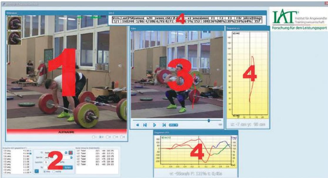
**FIGURE 1:** MAIN WINDOW FOR THE MEASUREMENT: 1) LIVE VIDEO PREVIEW WITH TEMPLATE DEFINITION FOR TRACKING (UPPER LEFT), 2) ATTEMPT SETTINGS FOR DATABASE (EXERCISE, NAME, LOAD, SET, REPS), 3) VIDEO PLAYBACK AFTER TRACKING WITH 4) FREE ADJUSTABLE DIAGRAMS AND TABLES WITH BIOMECHANICAL DATA
