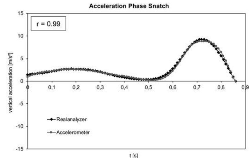
**FIGURE 3:** EXAMPLE OF COMPARISON OF VERTICAL ACCELERATION FROM ACCELEROMETER AND REALANALYZER FOR ACCELERATION PHASE IN SNATCH
