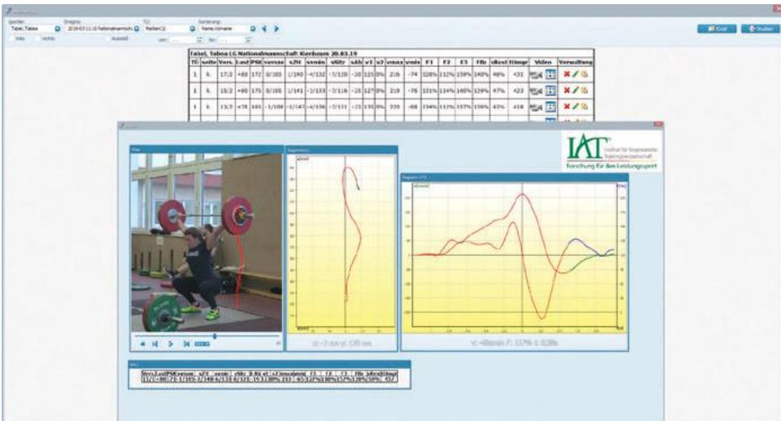
**FIGURE 2:** DATABASE OF REALANALYZER WITH OVERVIEW OF BIOMECHANICAL PARAMETERS (BACKGROUND) AND LOADED ATTEMPT WITH VIDEO, DIAGRAMS AND TABLE (FOREGROUND)
