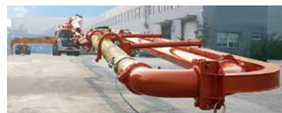
Pump Truck Boom Fatigue Test
