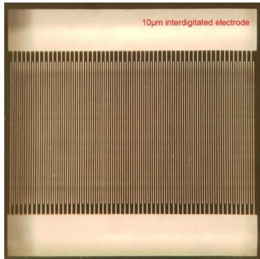
10  $\mu\text{m}$  interdigitated capacitor
