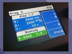
Each program can have several spinning steps with different speeds, accelerations and spinning times per step.
