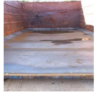
Replacing cross bearers/floor (opportunity to replace with better materials?). Pressed steel channel full of debris which has entered where the floor was holed above the bearer and rammed in by compaction
