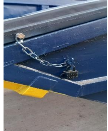
Example, enclosed skip with stabilising 'wedges' fitted to reduce the risk of the skip 'nose-diving' when loaded on a slope (provided the skip is facing the correct way)
