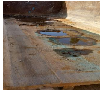
Replacing cross bearers/floor (opportunity to replace with better materials?). Pressed steel channel full of debris which has entered where the floor was holed above the bearer and rammed in by compaction
