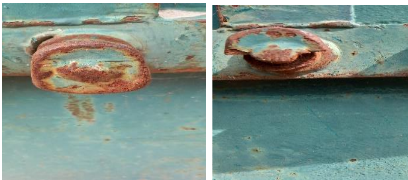
Examples of damaged and worn skip lifting lugs. In general, it is preferable to replace a skip lug with a forged type in lieu of a fabricated lug
