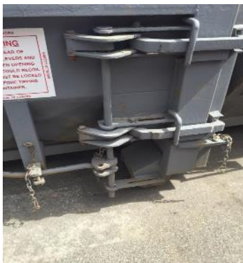
Example of a compaction container latching mechanism. Release lever is secured by a pin on a chain (to prevent its loss)
