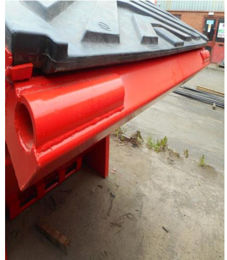
small skip refurbished - new tipping bar detail
