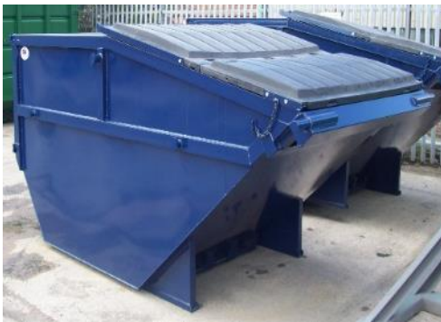
Example, enclosed skip with stabilising 'wedges' fitted to reduce the risk of the skip 'nose-diving' when loaded on a slope (provided the skip is facing the correct way)
