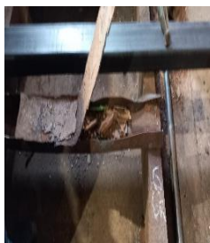
Replacing cross bearers/floor (opportunity to replace with better materials?). Pressed steel channel full of debris which has entered where the floor was holed above the bearer and rammed in by compaction
