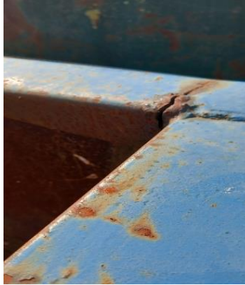
Two examples: container with bowed sides and tearing at the headboard
