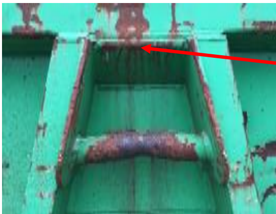
Collision marks on headboard cross tube, the upper protection plate has provided the tube with the required support
