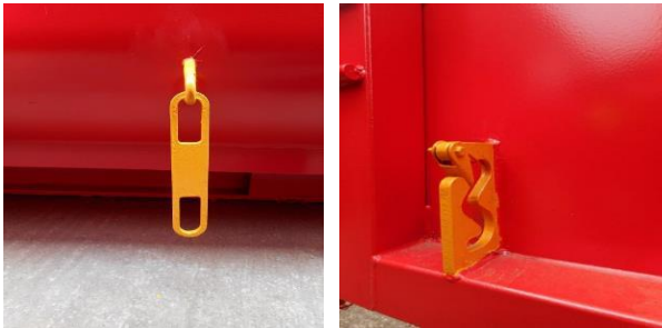
Door retaining loop and labyrinth/retaining plate (chain systems are not recommended)
