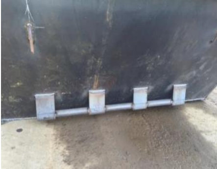
small skip refurbished - new tipping bar detail
