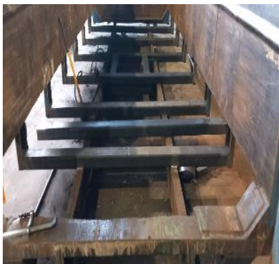
Damaged and holed floor with outline of bearers visible, and replaced floor
