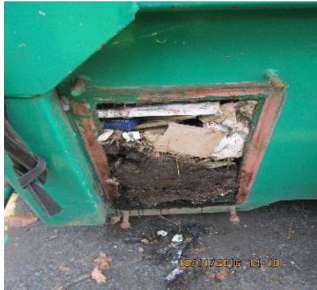
Two examples of debris trapped at the cylinder area (behind the compactor ram).
