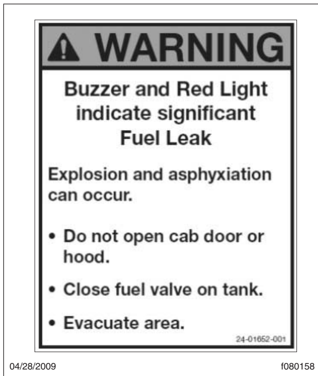
Fig. 16.5, Exterior Warning Sticker
