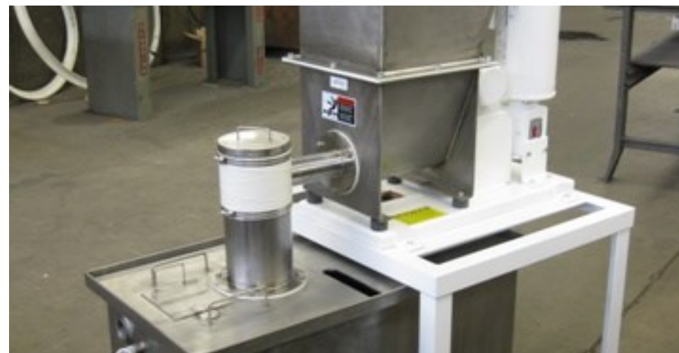
LOSS IN WEIGHT FEEDER
