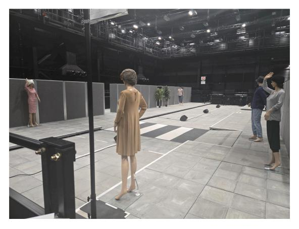
Each section of the configurable street contains sensors, and each section can be adjusted to introduce bumps or slopes for measuring responses in experiments (photo: G Byatt)
