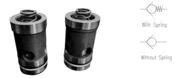
Check valves or non-return valves are designed to allow oil flow through them in only one direction and block in opposite direction. The unique flange locking design facilitates superior performance and zero leak. The valve may also be used without flange for replacement purposes. These valves are ideal for high flow applications and are available without spring (0 bar cracking) or standard 1.5bar cracking pressures.
