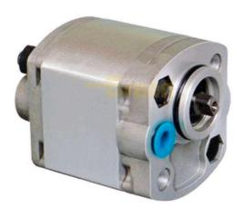
The CBK type fixed gear pumps are unique pumps with suction port on rear side and pressure (delivery) port on the shaft side. These are external gear pumps that use meshing of gears to pump fluid by displacement. The CBK pump find usage in equipments that use sandwich manifolds based hydraulic power-pack viz. car parking systems, fork-lifts, tipper and garage equipment/ vehicles.
