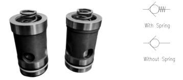
Check valves or non-return valves are designed to allow oil flow through them in only one direction and block in opposite direction. The unique flange locking design facilitates superior performance and zero leak. The valve may also be used without flange for replacement purposes. These valves are ideal for high flow applications and are available without spring (0 bar cracking) or standard 1.5bar cracking pressures.
