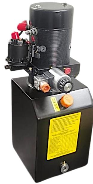
DC motor-driven hydraulic power-units, are commonly used in mobile applications where an electric battery provides the supply voltage. The electric motor is mechanically coupled to a hydraulic gear pump, which is then connected to a hydraulic circuit to perform the required function. They are commonly used in forklifts, garage trucks, scissor lifts, etc.
