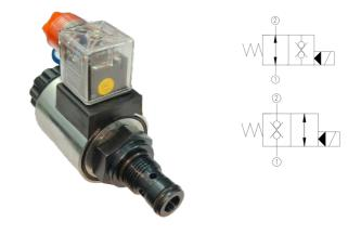
DHF 06 valves are solenoid-operated direct-acting poppet type 2-way and 2-position directional control valves that may be actuated by either DC or AC voltages to open or close the oil path. Once the coils are energised, the poppet opens/ closes and allows/ blocks oil flow from 1 to 2 or from 2 to 1 based on valve selection. The valve is designed for low pressure drop due to its design and is available in either 12/24VDC or 220VAC versions.
