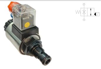
DHF 08 valves are solenoid-operated direct-acting poppet type 2-way and 2-position directional control valves that may be actuated by either DC or AC voltages to open the oil path. Once the coils are energised, the poppet opens and allows free flow from 1 to 2 or from 2 to 1 based on application requirements. The valve is designed for low pressure drop due to its design and is available in either 12/24VDC or 220VAC versions.
