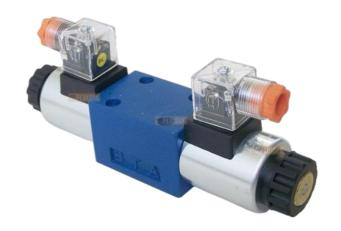
Directional Control Valves (DCV) are spool type valves used in hydraulics to change the oil flow direction using electric solenoids. These valves use wet-pin solenoids in AC or DC voltages and are used for vertical stacking valve assemblies. A variety of spool configurations including 4-pos/3-way and 4-pos/2-way are available with 12, 24VDC and 220VAC. The valves meet the requirement of CETOP3 mounting interface (ISO4401) and are compatible with equivalent valves of other manufacturers.
