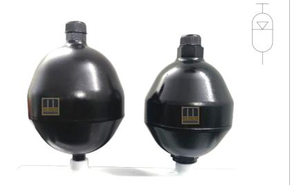
FAD is a hydro-pneumatic accumulator used to store liquid under pressure. A flexible membrane or diaphragm is fitted into the body to separate the nitrogen and oil chambers. An inert gas like Nitrogen is charged into the port G1 through a pressure valve to a pressure P0. As the diaphragm expands, it fills the complete volume of the accumulator body V0.
