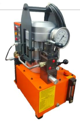
The Jack Power-Unit (FJPU) is a portable hydraulic power unit designed to lift heavy loads using either a single- or double-acting hydraulic jack. It features a robust, two-stage radial piston pump connected to an external motor, making it ideal for demanding, high-pressure applications. This compact unit is designed for portability, with a lightweight, single-phase electric motor and a carrying handle and comes standard with a control panel, pendant, and cooler.
