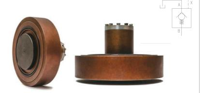
Pre-fill valves are check valves with hydraulic (pilot) release function. They are also referred to as exhaust valves and are generally installed between a cylinder and oil reservoir in hydraulic presses and injection moulding machines where high speed operation is required. The use of these valves enables the manufacturer to use a smaller capacity pump and motor and at the same time achieve the expected cycle time of the equipment.
