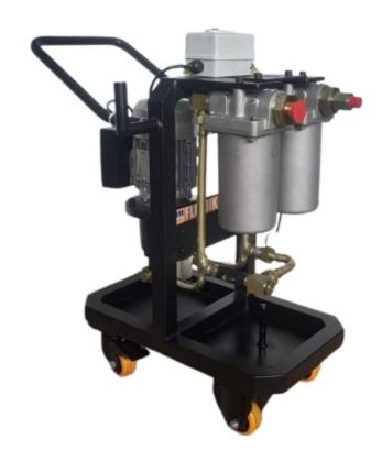
Hydraulic oil filtration trolley type FTR-1 is a single stage filtration unit that is portable and designed to clean and purify hydraulic oils by removing contaminants present in oil. These trolleys are essential for maintaining the health and longevity of hydraulic systems by ensuring that the oil remains within specified cleanliness standards and is recommended to be used either when filling oil from a barrel into the tank/ reservoir or periodically filter the oil in the system.
