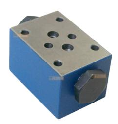
Sandwich type double pilot operated check valves (DPOCV) or sandwich isolator valve are used in hydraulic circuits for leak free closure of A & B ports for long periods of time. These valves are designed as internally piloted-to-open using pressure signal from opposite actuator port. The valves meet the requirement of CETOP 3 mounting interface (ISO4401) and used in vertical stacking assemblies.
