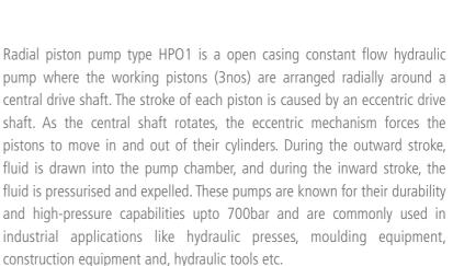
Use of open design pump makes it possible to reduce the size of power unit and these pumps are light weight and also economical when compared with other designs.
