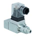
PSB pressure switches are electro-hydraulic type switches rated up to pressures of 700bar. These piston type switches are used to trigger electrical signal when a set pressure is achieved and can be configured as either NO or NC type. Designed for rugged and trouble free operation, these switches are available as sub-plate or line mounted versions (except 700bar). The standard non-LED plug-in connectors as per DIN 43650/ ISO 4400 are provided as standard with the product.
