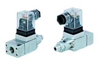
PSB pressure switches are electro-hydraulic type switches rated up to pressures of 700bar. These piston type switches are used to trigger electrical signal when a set pressure is achieved and can be configured as either NO or NC type. Designed for rugged and trouble free operation, these switches are available as sub-plate (4-bolt or 2-bolt) or line mounted versions. The standard non-LED plug-in connectors as per DIN 43650/ ISO 4400 are provided as standard with the product.
