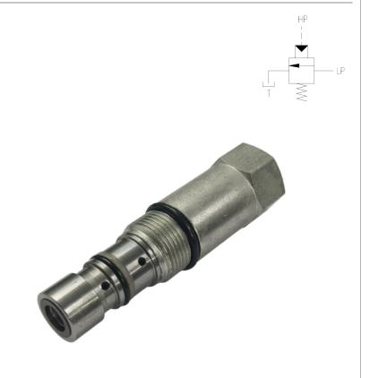
Pump unloading valve type PUV06 is crucial in high-low hydraulic circuits to efficiently manage system pressure and flow. Its primary purpose is to bypass the flow from the high-flow pump back to the tank when the system pressure reaches a predetermined set point, thereby "unloading" the pump. This unloading action significantly reduces the power required from the electric motor driving the high-pressure pump, as it no longer has to work against full system pressure and flow.
