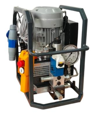
FTW EXT is a electrically operated hydraulic torque wrench power-unit/pump designed for working in harsh industrial environments. These are compatible with a variety of torque tools and can be operated up to 700bar pressure. Rugged yet light weight in construction, the power-unit is protected by an enclosure with an air-oil cooler as standard to meet higher duty cycle requirements.
