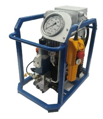
FTW EXT is a electrically operated hydraulic torque wrench power-unit/pump designed for working in harsh industrial environments. These are compatible with a variety of torque tools and can be operated up to 700bar pressure. Rugged yet light weight in construction, the power-unit is protected by an enclosure with an air-oil cooler as standard to meet higher duty cycle requirements.
