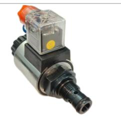
DHF 08 valves are solenoid-operated direct-acting poppet type 2-way and 2-position directional control valves that may be actuated by either DC or AC voltages to open the oil path. Once the coils are energised, the poppet opens and allows free flow from 1 to 2 or from 2 to 1 based on application requirements. The valve is designed for low pressure drop due to its design and is available in either 12/24VDC or 220VAC versions.
