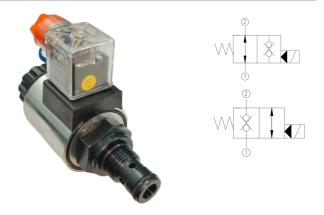
DHF 06 valves are solenoid-operated direct-acting poppet type 2-way and 2-position directional control valves that may be actuated by either DC or AC voltages to open or close the oil path. Once the coils are energised, the poppet opens/ closes and allows/ blocks oil flow from 1 to 2 or from 2 to 1 based on valve selection. The valve is designed for low pressure drop due to its design and is available in either 12/24VDC or 220VAC versions.
