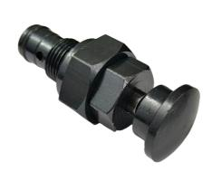
DHFM 06 valves are manual operated direct acting poppet type directional control valves that may be actuated by a spring return push knob to open the oil path. These are normally closed (NC) valves that are ideal for applications where emergency pressure release functions are required. When actuated, the valve allows oil to flow freely from port 2 to 1 and in closed position, the flow path is blocked in both directions.
