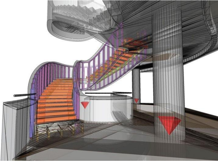
Figure 5. Structural/architectural model of one of the stairs created in Rhino-Grasshopper (Fjmt, 2025)
