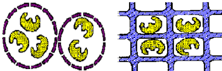
Figure 5. Microencapsulation and Cage-type immobilization method (Chang, 1976).
