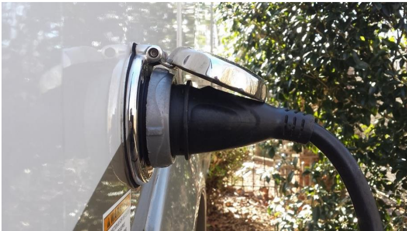
Fig 1.7: Shore power cord which is connected to a RV.[10]
