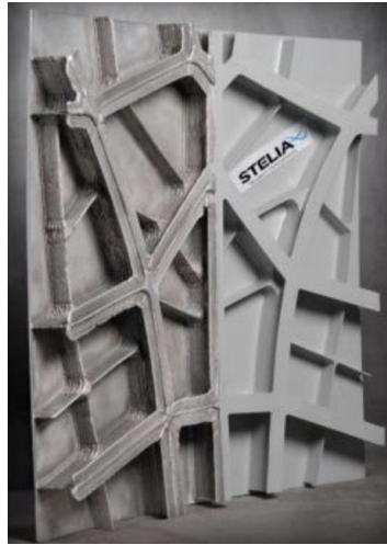
Figure 12. Body panel manufactured by additive manufacturing (Özsoy et al., 2020).
