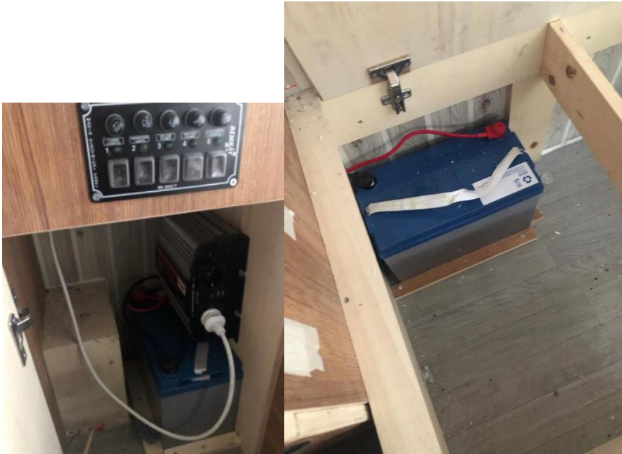
Fig 1.4: Batteries which are installed in a RV in Başkent Caravan.
