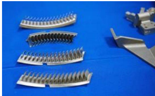
Figure 11. Stator to be used in Pratt Whitney jet engine bombardiers manufactured by additive manufacturing (Özsoy et al., 2020).
