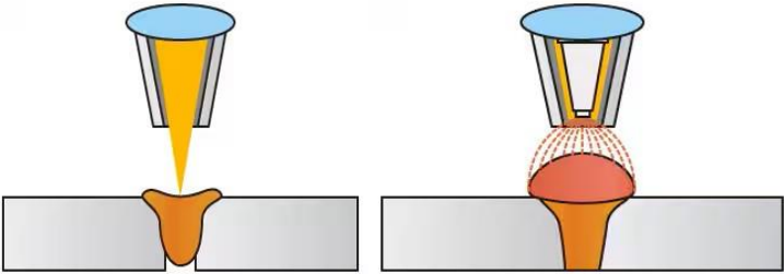
Figure 1. Laser Welding on the Left, Hybrid Welding Schematic on the Right.
