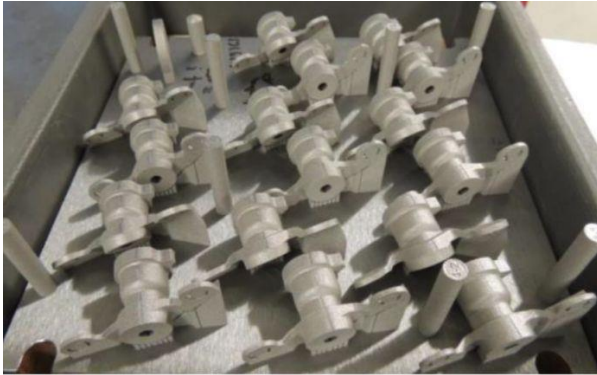
Figure 9. Borescope eye and tensile sample manufactured (Bamberg et al., 2015).
