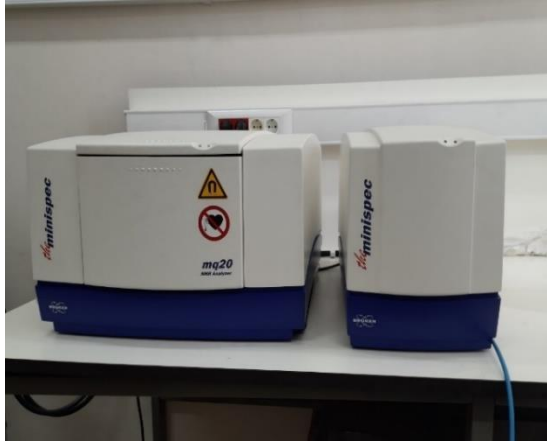
Figure 1. Bruker Minispec mq20 TD-NMR (20MHz-0.5Tesla)
