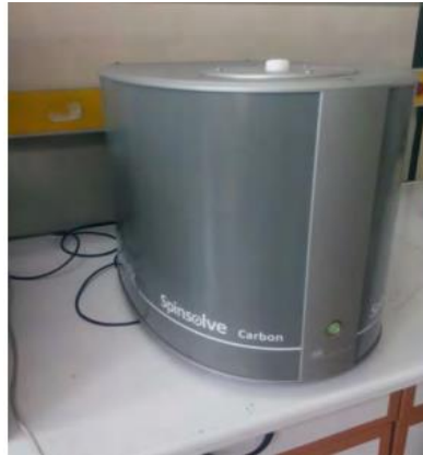
Figure 2. Magritek Spinsolve NMR (42MHz-1Tesla)
