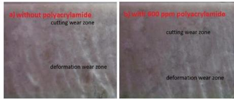
Figure 13. (a) Cutting surface without polyacrylamide solution, (b) cutting surface with polyacrylamide solution (600 ppm) (Hu et al., 2016)
