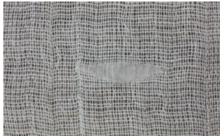
(a) Defect 1. Foreign material.
