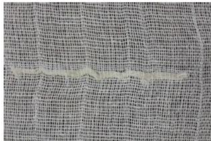
(b) Defect 2. Weft accumulation-1.
