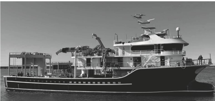
Figure 5. Cranes are installed on a purse seine vessel for operating power blocks, hoisting fishing gear, and performing auxiliary lifting tasks. Spreader and boom masts are not fitted on the decks of this type of vessel.
