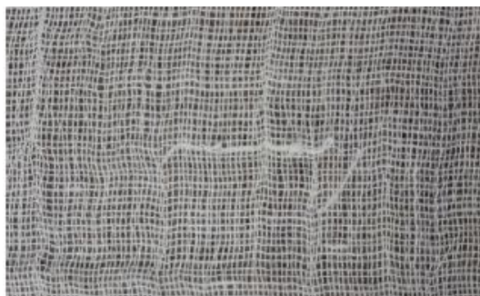
c) Defect 3. Weft accumulation-2.
