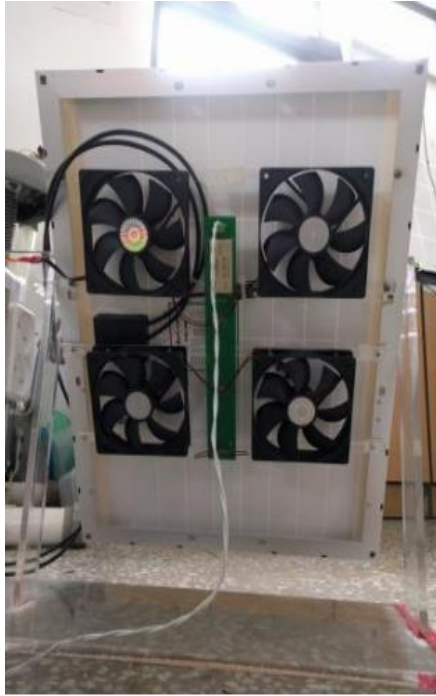
Fig. 8 Rear view of solar panel with four cooling fans
