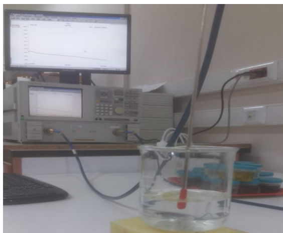
Figure 2. Agilent Network Analyzer (VNA) and Dielectric Kit.
