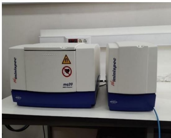
Figure 1. Bruker Minispec mq20 TD-NMR (20MHz-0.5Tesla)
