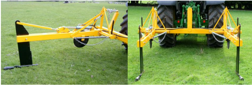
Figure 3. Mole plough and its attachment to the tractor (Anonymous 2025d)
