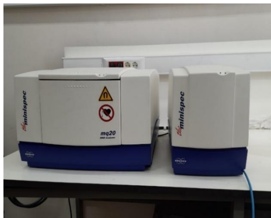
Figure 1. Bruker Minispec mq20 TD-NMR (20MHz-0.5Tesla)
