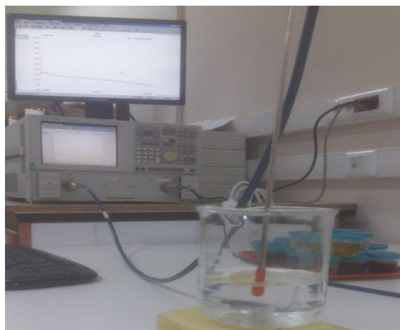
Figure 2. Agilent Network Analyzer (VNA) and Dielectric Kit.
