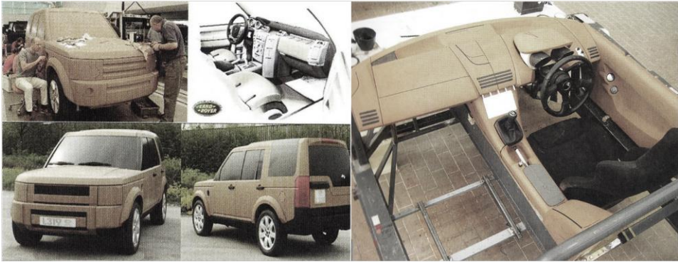
Figure 11. Digital clay scanning & CNC clay modeling phase (Tovey, 2012).
