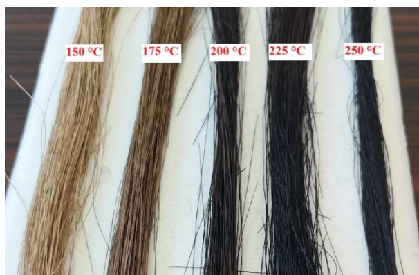
Fig. 3 Color change of untreated and PA-BA-pretreated then stabilized hemp fibers
